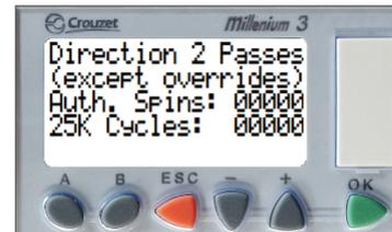
This screen gives statistics about how many times direction 2 was activated and cycled. Since there is a limit to how many counts can be displayed, after 25000 cycles the first counter resets and adds to the second counter.
