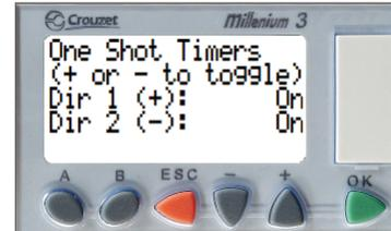
This screen allows for the two one-shot timer settings to be enabled or disabled. This setting prevents access control from holding open a direction on the standard direction inputs. Toggle Direction 1 by pressing + and Direction 2 by pressing -. This should be set to "On" in almost every installation.
