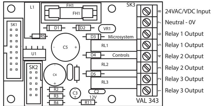
The coin mechanism can be configured to give different outputs in different circumstances, but for the purposes of connecting to a turnstile or gate, only Relay 1 is used. Interfacing the VAL 343 to the turnstile's logic controller is fairly basic. 3 wires are ran from the VAL 343 to the 6500 Series Control Head. This device should be wired as an access control device per the wiring diagram. Specifically, the device connects as follows:
