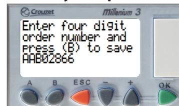
This screen should only appear when first set up in the factory or if something occurs to totally reset the logic controller. If this manages to occur and the order number (if known), enter it as a value then press B to save.
