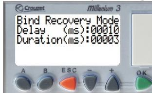
The motorized gate logic includes a function which briefly reverses the motor in the event of a mechanical bind against the locking bar. The delay before this occurs and the duration of reverse time can be adjusted here. The default delay is 10 ms and the default duration is 3 ms. These settings shouldn't be altered without guidance from tech support.
