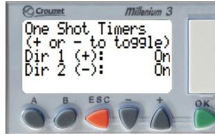
This screen allows for the two one-shot timer settings to be enabled or disabled. This setting prevents access control from holding open a direction on the standard direction inputs. Toggle Direction 1 by pressing + and Direction 2 by pressing -. This should be set to "On" in almost every installation.
