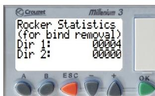
This screen displays how many times the motor rocked the arm in the event of a mechanical bind for each direction. This information may be useful to technical support.
