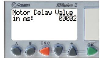
This screen allows for the modification of the setting which adds a delay after the motor moves before it can move in the opposite direction. This is mainly to protect the logic controller from shorting out the motor. This value can scale from 1 ms to 60 ms. Default value is 2 ms.
