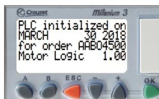
This screen displays when the PLC was initiated, the order number it was activated for (except for any revision suffixes which are not needed for order lookup), and the PLC software version.
